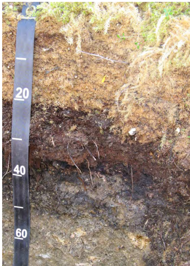
Figure 3-3: Soil profile in Alaska that has a histic epipedon extending to a depth of about 38 cm. The upper 20 cm is fibric soil material that has a high content of Sphagnum overlying more decomposed organic soil material. Scale is in cm. (Photo courtesy of Dr. David Weindorf)
