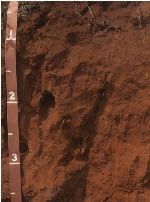
Figure 3-19: Profile of an Oxisol in Jamaica that has a highly weathered red, clayey oxic horizon below a slightly darkened ochric epipedon. Scale is in feet.
