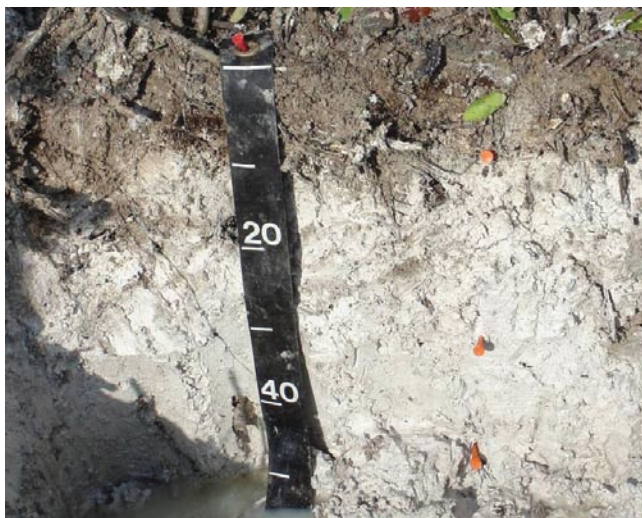
Figure 35.—Indicator F10 (Marl). In this profile, marl begins at a depth \leq 10 cm of the soil surface. The scale is in cm.
