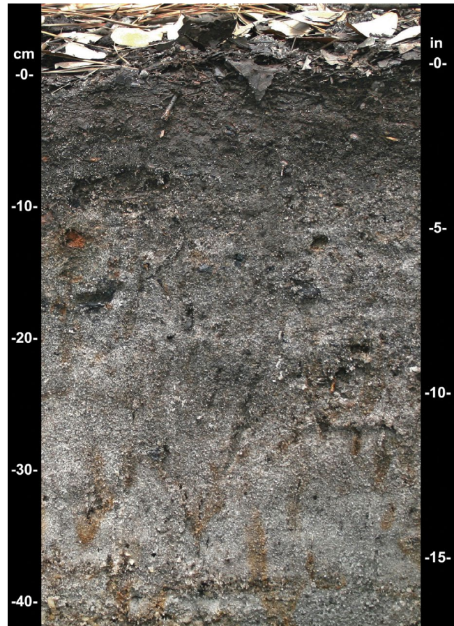
Figure 22.—Indicator S5 (Sandy Redox). This soil meets the requirements of indicator S5, having a matrix chroma of 2 or less and at least 2 percent redox concentrations starting at a depth of about 10 cm.
