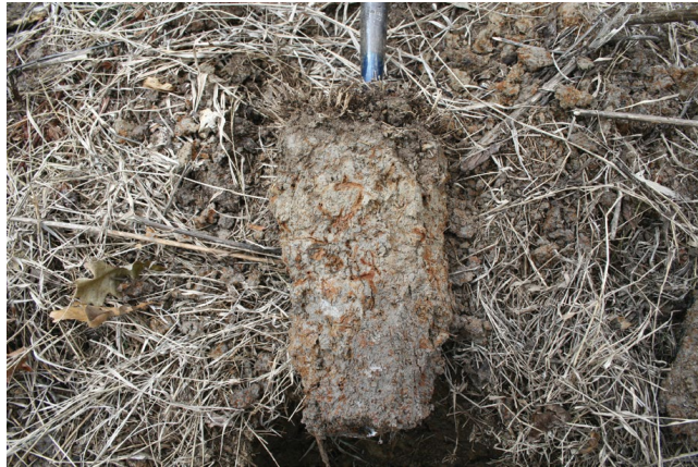
Figure 45. —A depleted matrix with value of 4 or more and chroma of 2 or less. Redox concentrations occur as soft masses and pore linings.
