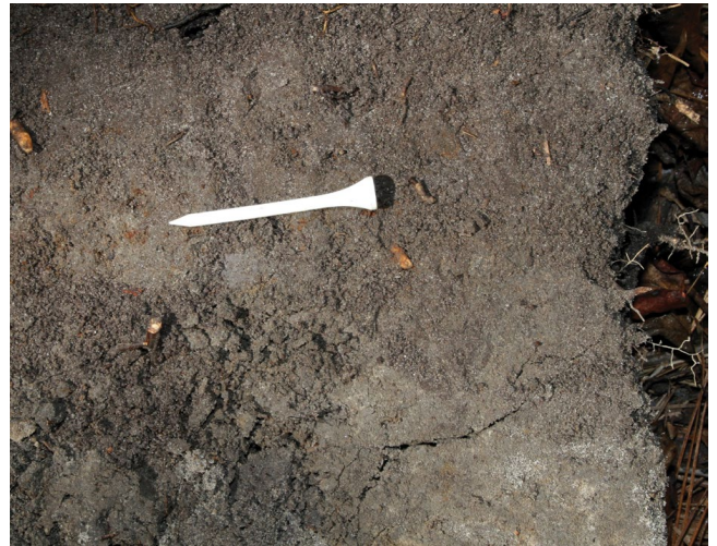
Figure 32.—Indicators F6 (Redox Dark Surface) and F7 (Depleted Dark Surface). An example of both depletions and concentrations in a dark matrix.
